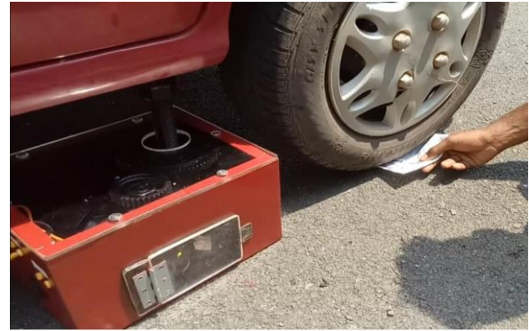
Figure 8: Car-jack doing actual lift testing
