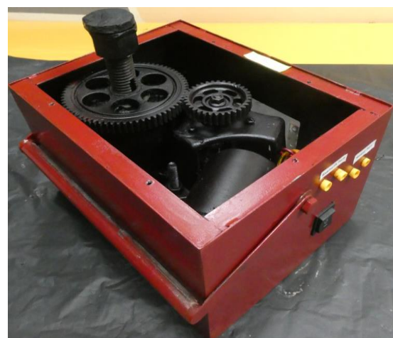
Figure 3: Car-jack in the metal casing
